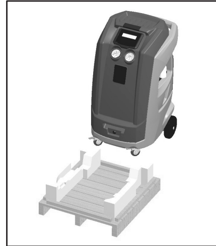
Fig. 12: Lowering unit from the pallet
