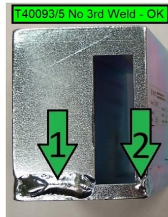
**The presence of a third weld indicates replacement is needed.**
