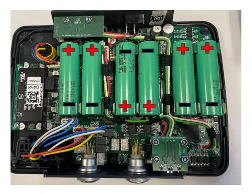
After installing the new batteries and securing the rear casing, make sure to check the red stop button on the front, as it may have been pressed while the tool was turned over during maintenance.
