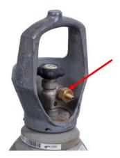
28. Connect the hose to the cylinder adapter. Spanner width: 14 mm. Torque: 16 ... 18 Nm, max. 20 Nm.
