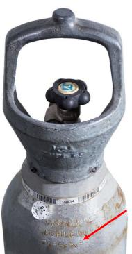
a) Mark the location of the outlet valve on the refrigerating agent cylinder.
