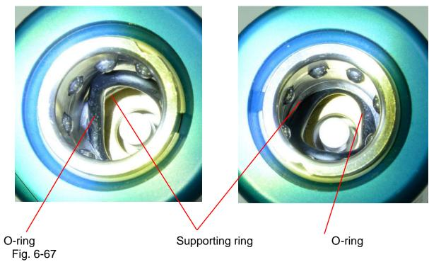
7. Push the O-ring further into the groove until the O-ring is seated evenly in the groove as shown in the figures.
