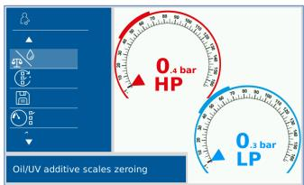
Fig. 6-53 Oil/UV additive scales zeroing
