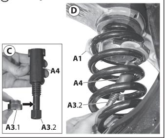
16. Rotate the pressure plate with swivel bearing "A2" in the chassis spring upwards, and remove it. (Fig. 33)
