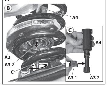
3. Insert the pressure plate with swivel bearing "A2" into the bottom section of the chassis spring. (Fig. 6)
