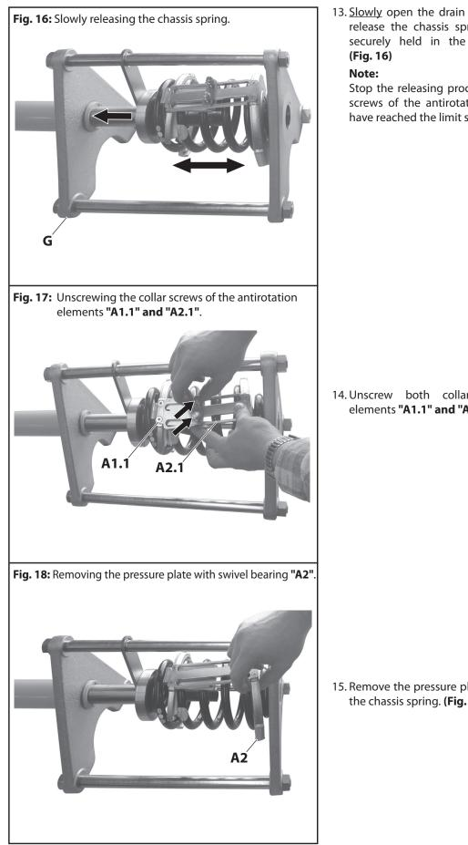
13. <u>Slowly</u> open the drain valve at the hydraulic pump and release the chassis spring to the extent that it is still securely held in the hydraulic clamping device **"G"**. **(Fig. 16)**
