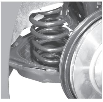
Rotate the pressure plate with catch "A1" in the chassis spring downwards, and remove it. (Fig. 35)
