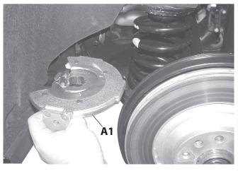
Fig. 36: Removing the spreader "E".
