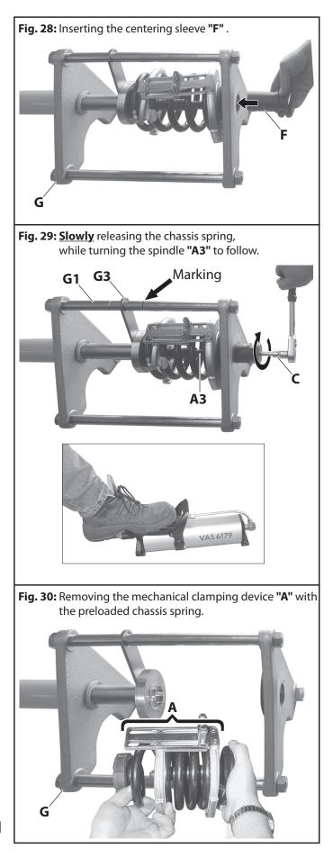
8. As required by the vehicle, insert centering sleeve "F" into the hydraulic clamping device "G" such that the flange of the spindle "A3" is guided in the centering sleeve "F". (Fig. 28)
