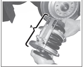
7. Insert the retaining wrench "D" completely into the upper pressure plate with catch "A1". (Fig. 10)
