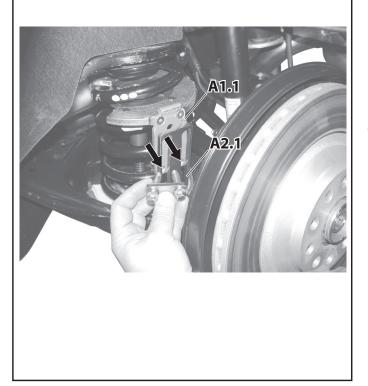
5. In order to be able to tension the different chassis springs to as small a dimension as possible, as many spring coils as possible must be tensioned.
