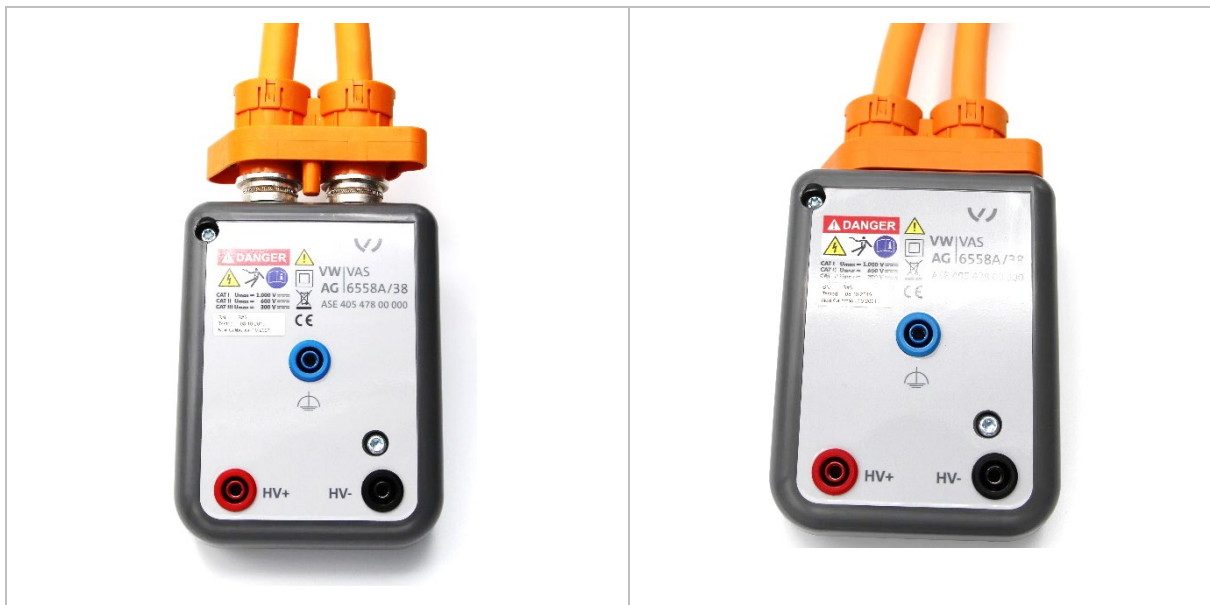
Fig. 3: Insertion position of the high-voltage cables
