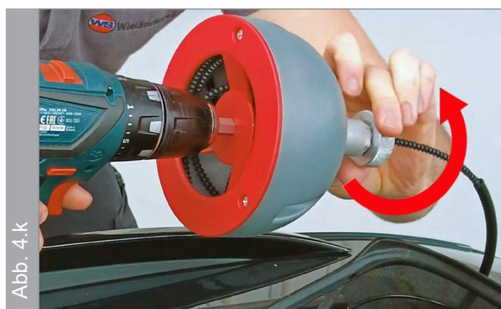
Now push the shaft back into the water drainage hose while turning it.
