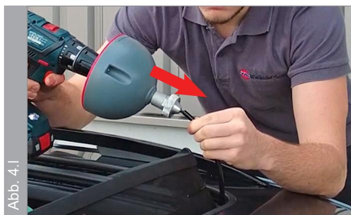
When cleaning is complete, pull the special shaft out of the water drain hose.
