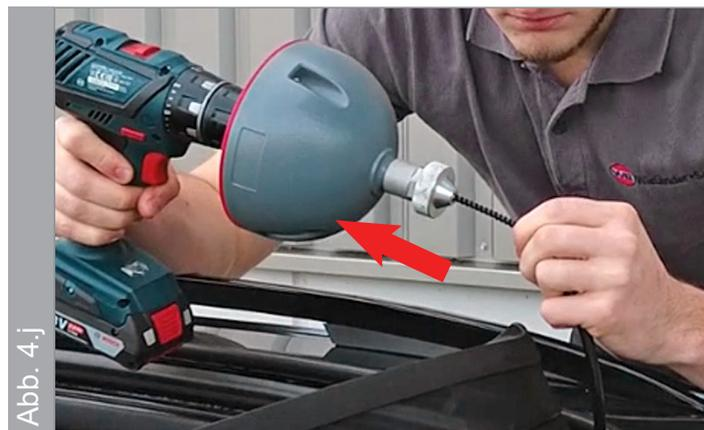
Close the tensioning device. Now the shaft again, under turn, insert into the water drain hose.
