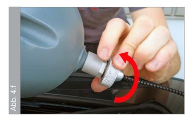
Hold the protective hose with one hand to guide the special shaft.
