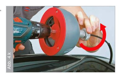
Now push the shaft back into the water drainage hose while turning it.
