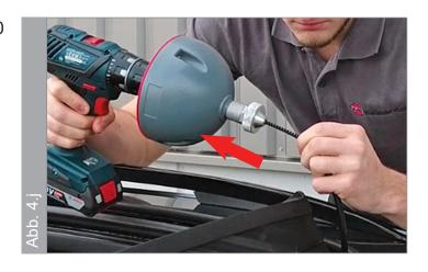
Close the tensioning device. Now the shaft again, under turn, insert into the water drain hose.
