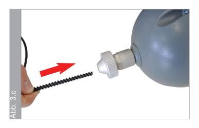
Push in the special shaft until the shaft is wound up to the protective hose in the receptacle.
