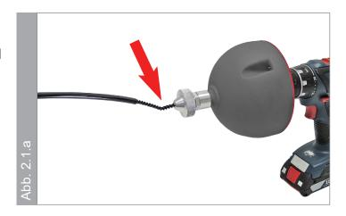
Before each new cleaning, check the special shaft for damage (kinks) and whether the protective cap is on the end of the shaft.
