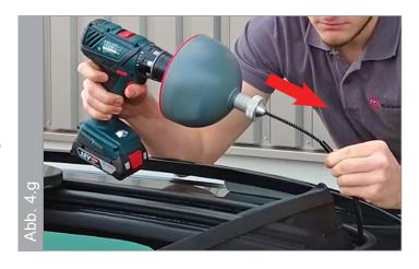
Screw the special shaft into the vehicle until the collet chuck reaches the protective hose.
