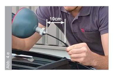
Tighten the clamping device only slightly by hand to lock the shaft in the cleaning aid.
