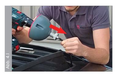
When cleaning is complete, pull the special shaft out of the water drain hose.
