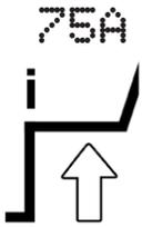
At the start of the welding process, the welding element (the stud) in the welding gun is raised using a lifting mechanism (lifting magnet). The activated start-up current is then used to generate a pilot electric arc.
